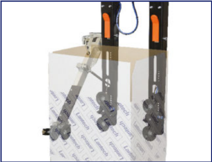
Square Case Erecting Six vacuum powered suction cups hold the blank in the correct position after it leaves the magazine. Both leading panels are held securely.
